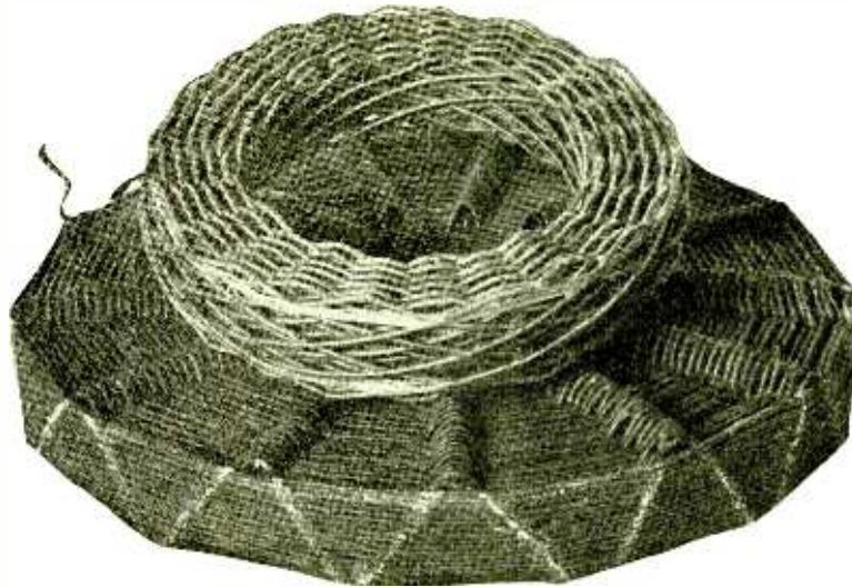
Fig. 7. Specimens of Duo-Lateral and Lattice Coils. Note the Track of the Zig-Zag Spacing Turn in the Lattice Coil.
