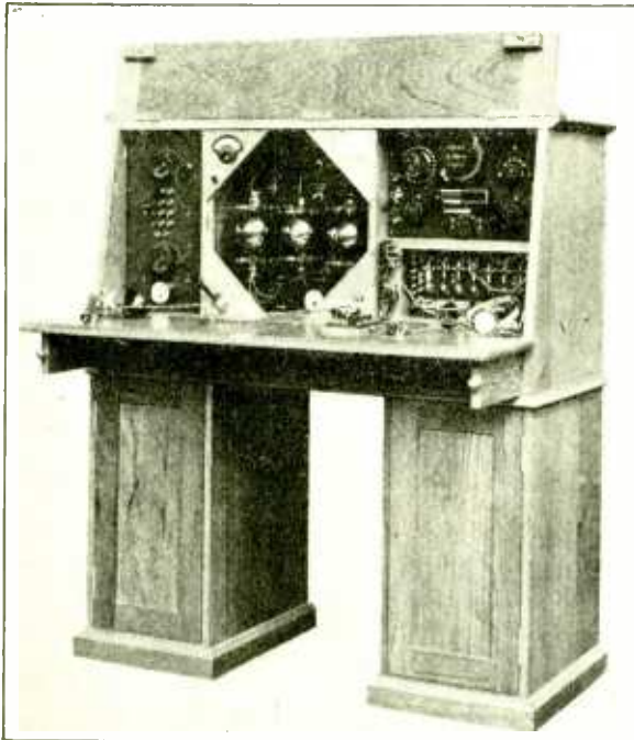
By Courtesy of Marconi Wireless Telegraph Co., Ltd. Fig. 92. Half-kilowatt Valve Transmitting Set for Wireless Telephony as Arranged by Marconi Wireless Telegraph Company, Ltd. The Transmitting Valves are Shown in the Center Panel and the Receiving Valves on the Right-hand Bottom Panel.
