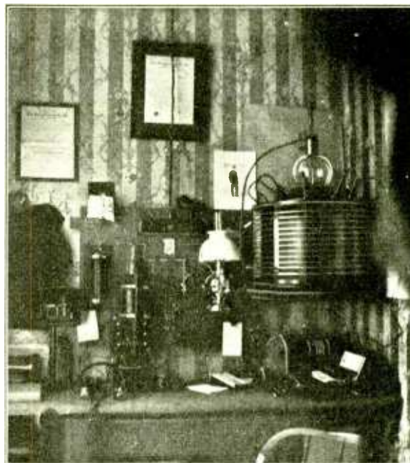
Station "A" One Year Later, Situated at Cape Cod. This is Quite an Improvement Over the Old One. Note the Size of the Helix and the Stationary Gap Inside the Glass Bulb. At First Glance This Looks Like a 50-Watt Vacuum Tube.
